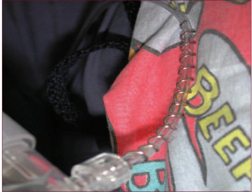
**Figure 3.** Sampling line with spring applied; it bends but does not kink.
