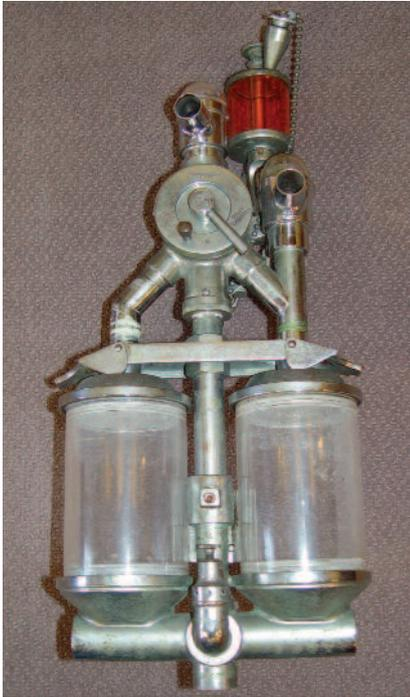
**Figure 5.** A Double Canister Circle Filter
